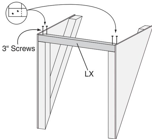
3. Attach the window header, LX, to the top of the brackets as shown. Fasten using four 3" screws.
