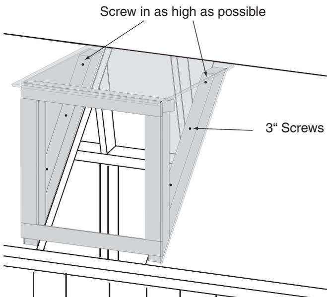
7. Center dormer over hole and attach using six 3" screws in the locations shown. Screws should be driven at a slight angle to be driven into the rafters.
