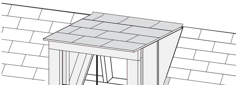
15. Using an exterior grade caulk, be sure to caulk all joints around the dormer including above and below trim and along the underside of the roof panel. Paint must also be applied to trim and siding.
