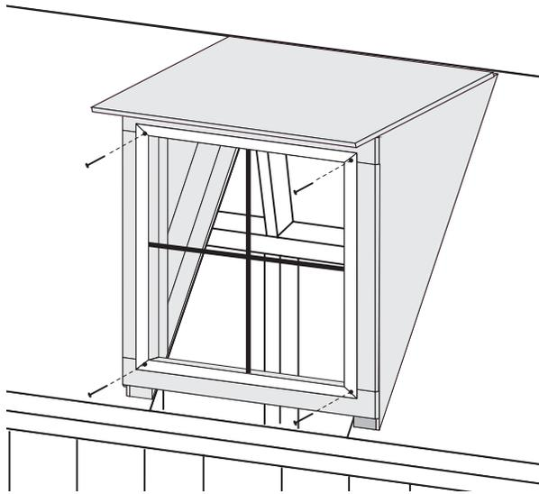
8. To attach window, center in the hole and fasten using four 1-1/4" screws in the pre-drilled corner holes.
